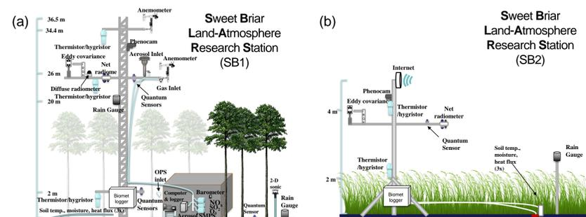
Figure 1. Schematic of the instrumentation at the (a) loblolly pine and (b) switchgrass eddy covariance towers.
